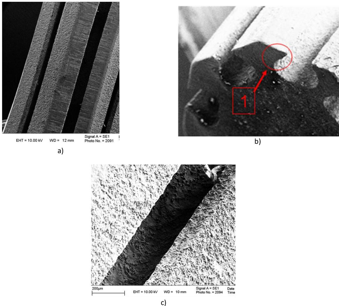
**Figure 3 - a) A top view of a prototype of a titanium implant with a developed surface in the form of a longitudinal channel with round shape macro-topography; b) side view of a prototype of a titanium implant with a developed surface in the form of a longitudinal channel with round shape macro topography; c) the increased surface of the longitudinal channel and the surface of the implant.**
