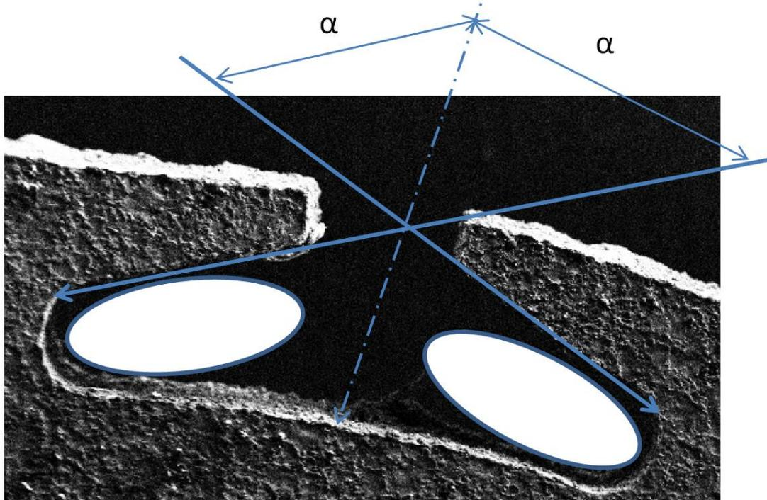
**Figure 2 – Ellipse zones that are the most difficult for coating of trapezoidal-shaped macropores**
