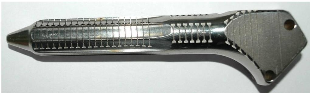
**Figure 1 – General view of the experimental sample of the endoprosthesis leg of the shoulder joint with a developed surface**
