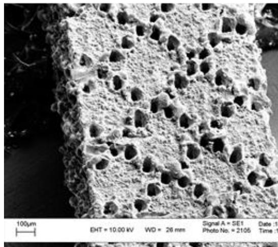
Figure 4 – The surface of area of the experimental sample formed by holes of cylindrical shape
